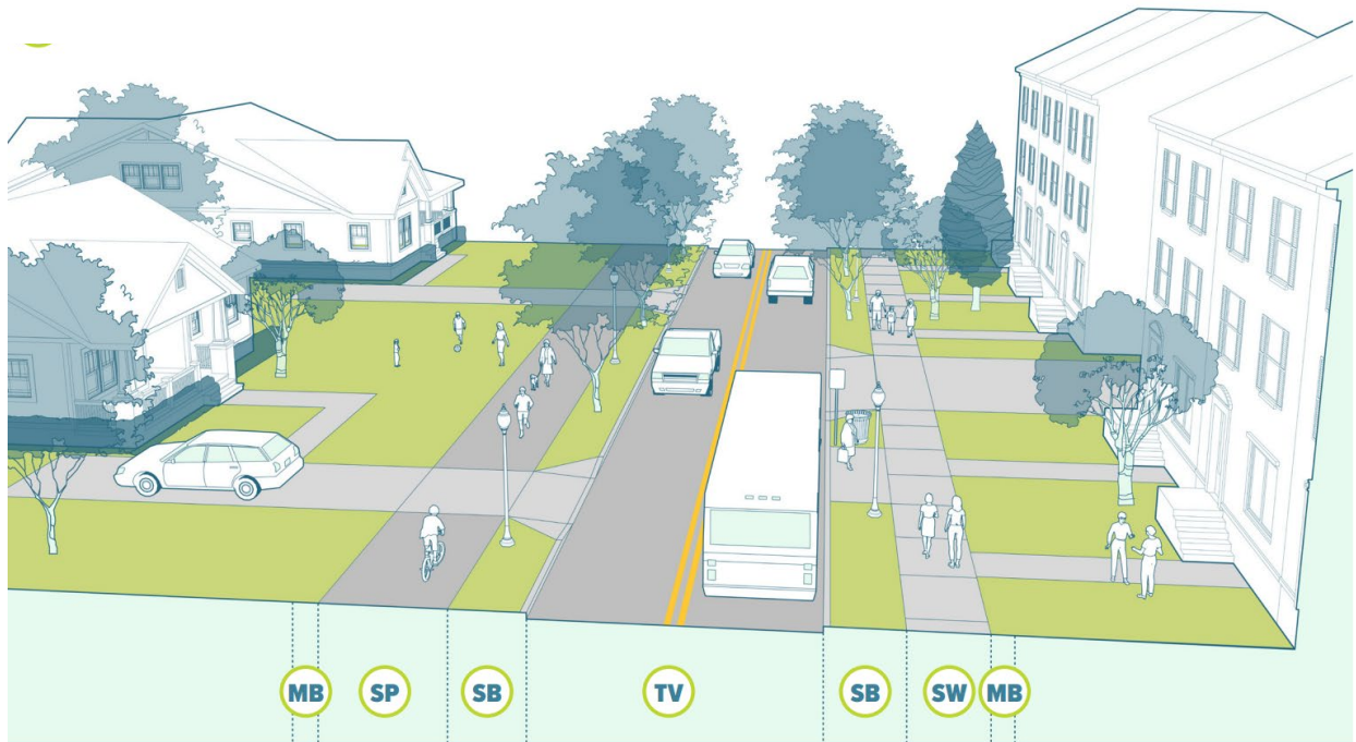
Figure 6: Neighborhood/Area Connector Cross-Section
